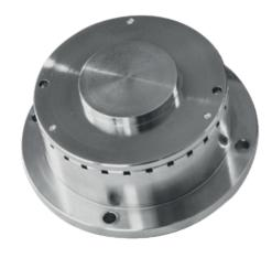
Optionally available die set with defined polished surface to investigate wall slip effect on rubber compounds. For complete measurement of the effect, the die set must be exchanged during the measurement.
