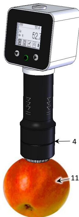
Fig. 7 Determination of the firmness of the pulp on fruit
