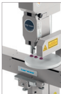
Laser-controlled positioning of O-rings
