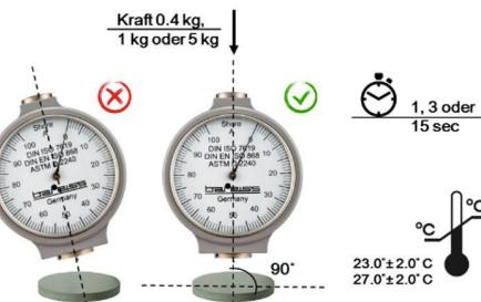
Room temperature, contact pressure and test time must be taken from the relevant standards and must be observed. If the plane-parallelism between the test specimen and the contact surface of the hardness tester is not kept and if there is a deviating contact pressure, measuring uncertainties may occur.
