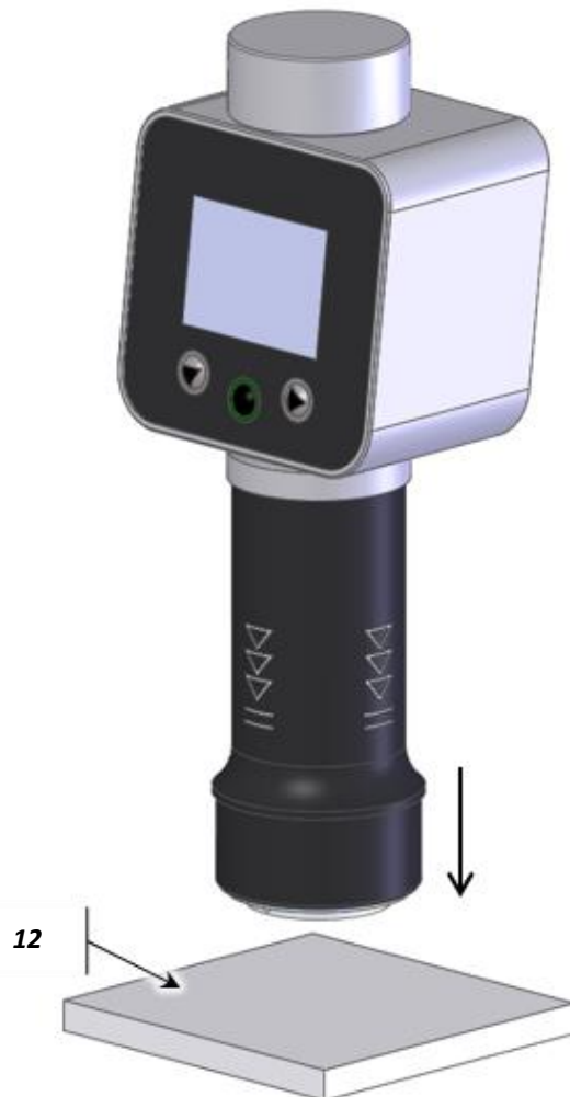
Fig. 13 Hardness testing for Shore 00, 000, 000 S
