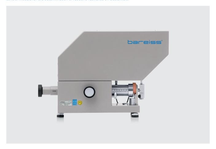
The rebound elasticity tester determines the flexibility of elastomers and similar materials, in a fully automatic manner, without operator influence. Thanks to the optional temperature control module, it also allows for measurements on heated test specimens to be performed. As a result, it offers information on the changes occurring in the elasticity of materials, under the influence of temperature.
