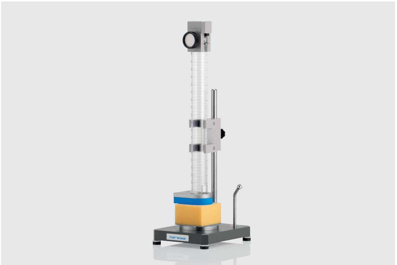
The elasticity of polymeric foam materials can be analyzed by measuring the rebound height of a ball after the free fall and impact on a test specimen.
