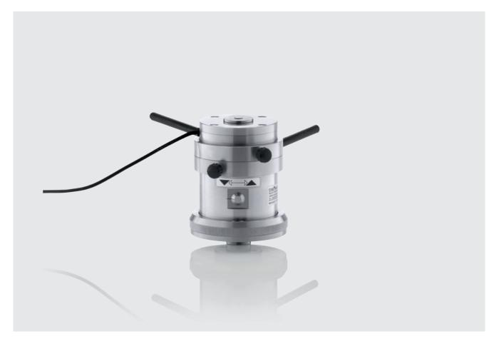
With the patented Kal-Rock, you can verify the penetration depth measuring device of your Rockwell hardness tester. With a resolution of 0.3  $\mu m$ , it controls the length measuring system of the hardness testers, under a maximum preload of 10 kg.
