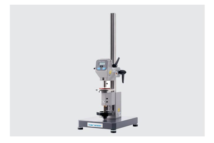
Our budget-friendly tester offers you the possibility to perform semi-automatic hardness tests with the methods IRHD M and IRHD N by means of interchangeable measuring devices- and all this with the same quality expected from Bareiss.
