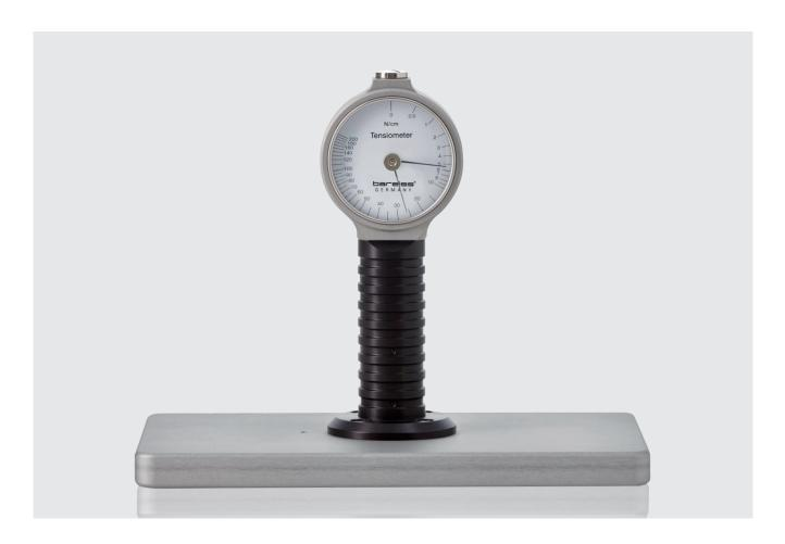
The Tensiometer measures the tension of wires and felts on running and stationary paper machines.
