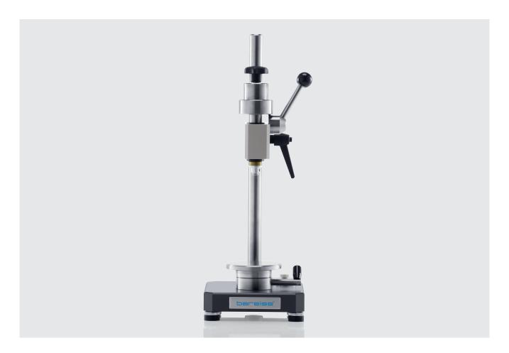
The test stand BS 61 II is used as additional equipment for analog HP or digital HPE III. With the support of the test stand, the user's influence on the measurement results is reduced.
