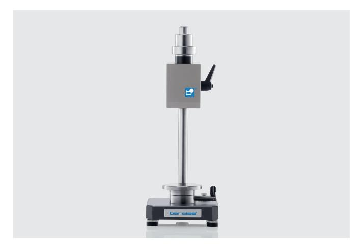
The automatic test stand BSA expands the application area of your Bareiss handheld hardness tester from mobile use to a stationary hardness tester in the laboratory. The BSA automatically lowers the hardness tester onto the sample with a constant lowering speed conforming to standards and provides the normative contact pressure with its total mass. With the available additional weights for different measuring methods you can flexibly adjust it.
