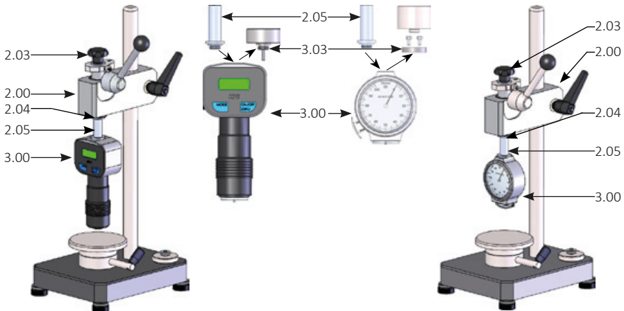
Fig. 3 Mounting the hardness testers Shore 00, Shore 000, Shore 000 S
