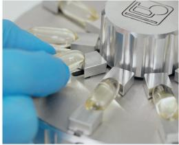
The Rotofix is the smart automation solution for hardness testing on multiple samples at the push of a button. In combination with the Gelomat, it offers the perfect entry point into automation.
